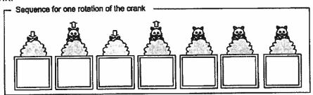
The toy designers wants the cat to move in and out of the box twice with each rotation of the crank and to remain out longer the second time.
